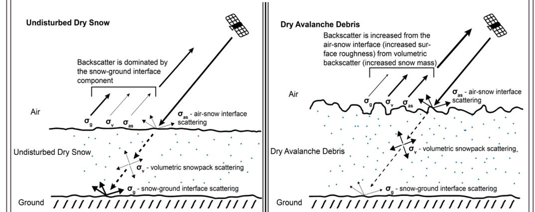
Figure 3: Simplified model of radar backscatter contributions for dry avalanche debris. Increases in surface roughness and snowmass are currently proposed as the primary contributors to increased backscatter for avalanche debris. Figure adapted from: Eckerstorfer and Maines (2015).
