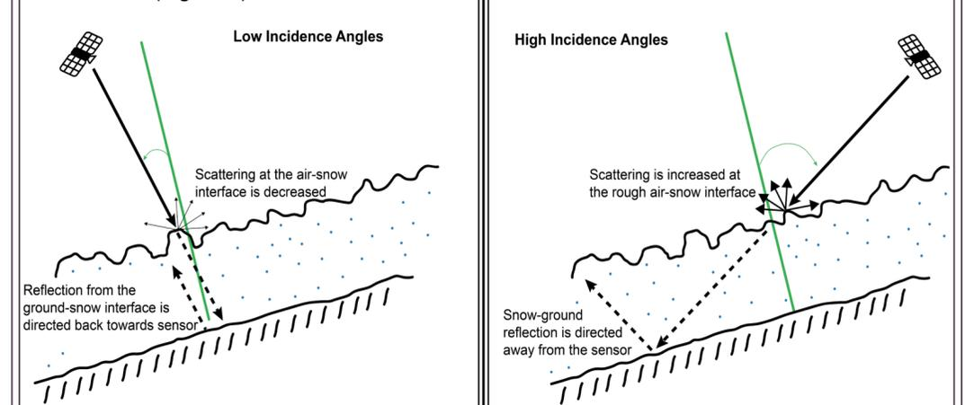
Figure 4: Idealized backscatter components for high and low incidence angles. Volumetric backscatter has been excluded for clarity.
