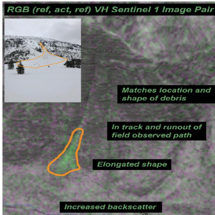
Figure 1: RGB image with reference S1 VH image in the red and blue channels and VH activity S1 image in the green channel. Green represents increases in backscatter and purple represents decreases. Inset field image courtesy of: Bridger-Teton Avalanche Center.
